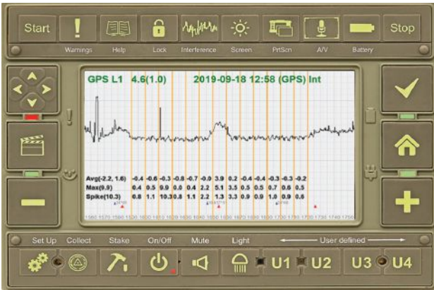
30 MHz-wide spectrum of the signal.
