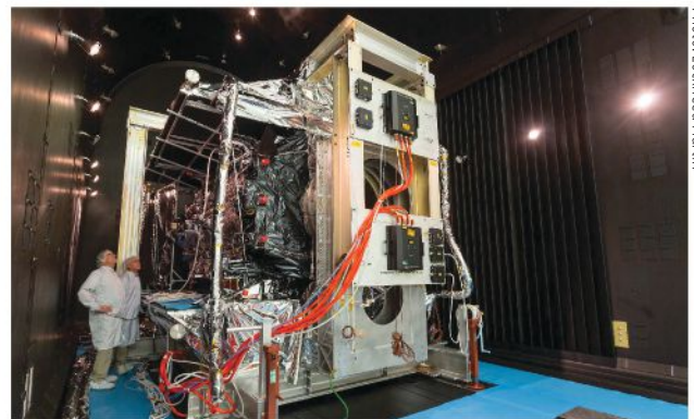
Thermal vacuum testing verifies that a satellite can operate in space's extreme environment.
