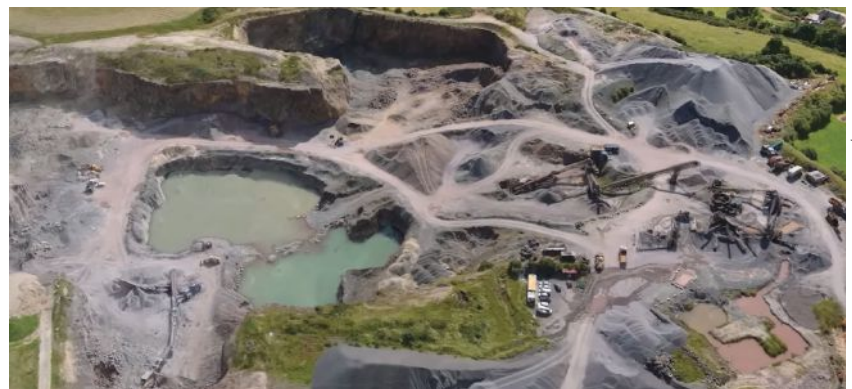
DRONES AID IN MANAGEMENT of complex, dynamic environments such as at this quarry in Ireland. Safety is also improved. This screenshot is from a fly-through animation generated using Pix4D Mapper software.
