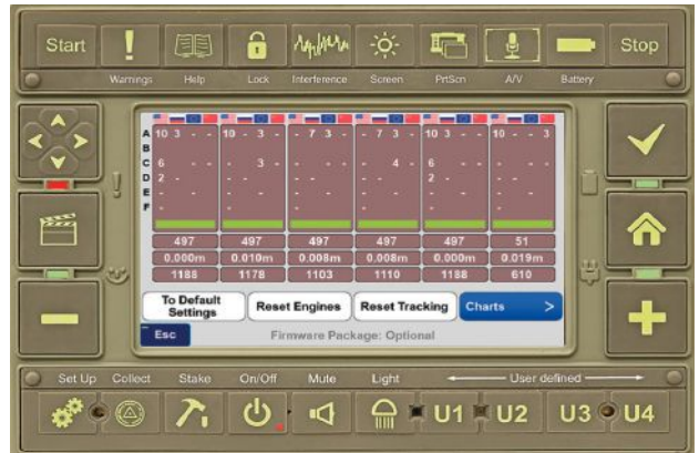
Six parallel RTK engines.
