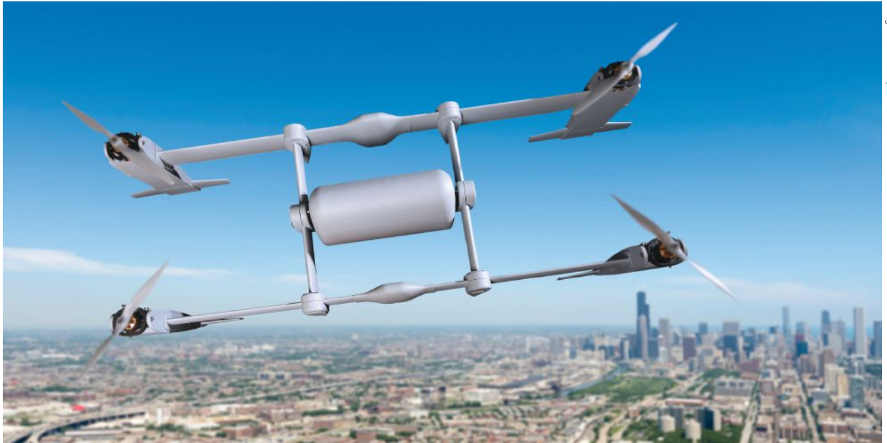
BELL'S APT 70 will be used as part of a NASA program in 2020. Bell aims to begin BVLOS tests in 2020, and begin commercial service soon after. The electric APT 70 can carry 70 pounds, cruise at 75 mph and cover 35 miles with a fully charged battery.
